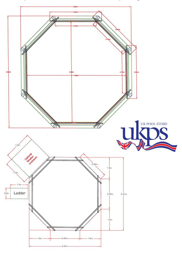
Minimum base size for this pool is 5.6m Square. This should be 100mm [4"] thick concrete. Ideally you can build the concrete base on top of sheet polystyrene insulation as this will provide added thermal insulation, so reducing any heat loss to the ground. Consider extending the base on one side to accommodate the landing area for the external ladder.
