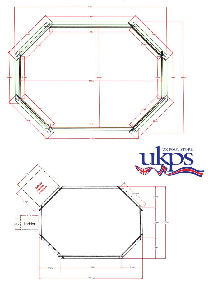
Minimum base size for this pool is  $8.0m \times 5.6m$ . This should be 100mm (4") thick concrete. Ideally you can build the concrete base on top of sheet polystyrene insulation as this will provide added thermal insulation, so reducing any heat loss to the ground. Consider extending the base on one side to accommodate the landing area for the external ladder.
