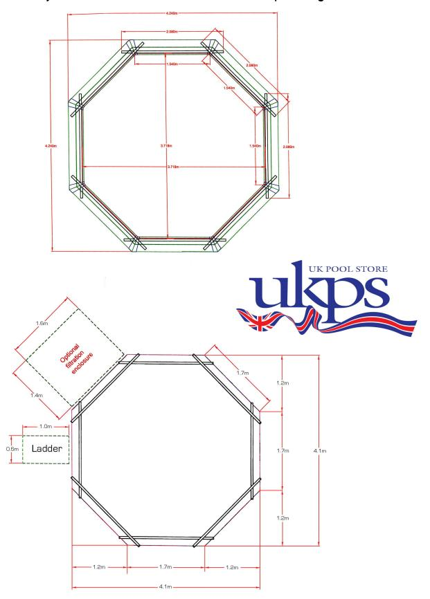
Minimum base size for this pool is 4.2m Square. This should be 100mm (4") thick concrete. Ideally you can build the concrete base on top of sheet polystyrene insulation as this will provide added thermal insulation, so reducing any heat loss to the ground. Consider extending the base on one side to accommodate the landing area for the external ladder.
