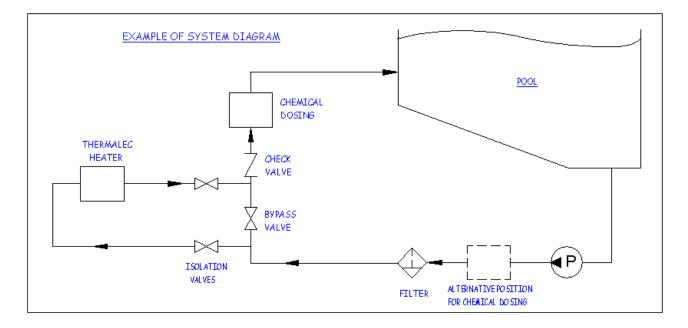
Chemical dosing systems should not be installed adjacent to the heater. If installed upstream of the heater it must be before the filter. If installed downstream, a check valve must be fitted to prevent backflow of chemicals when the filter pump is not operating. There should be a drop in level between the pipe leaving the heater and entering the dosing system.
